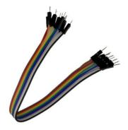
Jumper cables / wires are simply wires that have connector pins at each end, allowing them to be used to connect two points to each other without soldering. Jumper wires are typically used with breadboards and other prototyping tools to make it easy to change a circuit as needed. The colour variation of the wires can be used as advantage to differentiate between types of connections, such as ground or power.
