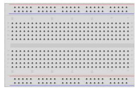
A breadboard is a plastic board with tiny holes in it which permit the easy insert of electronic components (transistors, resistors, chips, etc.) to prototype (build and test) an electronic circuit. The inside is made up of rows of tiny metal clips to hold the leads to be connected.
