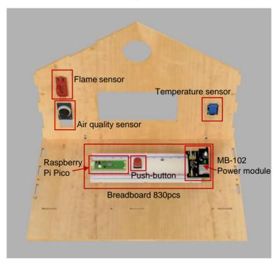
Place the Raspberry Pi Pico on the breadboard, along with the power module (MB-102) and the push button. The breadboard has an adhesive surface underneath, so make sure to peel off the protection layer and then place it on the base piece of the house.
