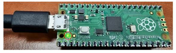
Press the Enter key and immediately the Pico's onboard LED will turn on.
