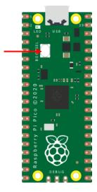
Step 3: Press the BOOTSEL button and hold it while you connect the other end of the micro-USB cable to your computer.
